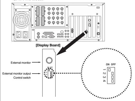
The distance between the DVR and external monitor should be measured then you can change the control switch on the back of the DVR accordingly. There are 4 level settings for the difference distances between DVR and Monitor so you can select which gives the best picture.
